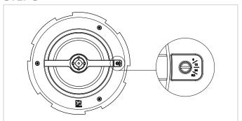
Using a flat head screwdriver, the power tap or low impedance selection can be made.
