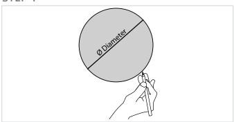
Cut a hole on the mounting location in the ceiling. Make sure the diameter is matching the cut-out measurement for the loudspeaker.
