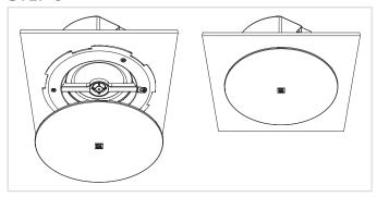
Attach the grill to the speaker by inserting the lips into the provided openings on the speaker baffle and rotate it over a partial turn (15°).
