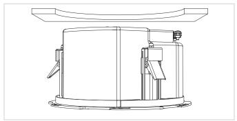
Make sure the spacing between the mouting surface and the clamp is bigger than the thickness of your ceiling plate. Insert the speaker until the clamps snap in place
